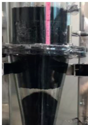
Fig. 5. Fluidization image of carbon nanotube agglomerates in 100-mm-bed-size fluidized bed at U_g = 0.0318 m·s -1 .
